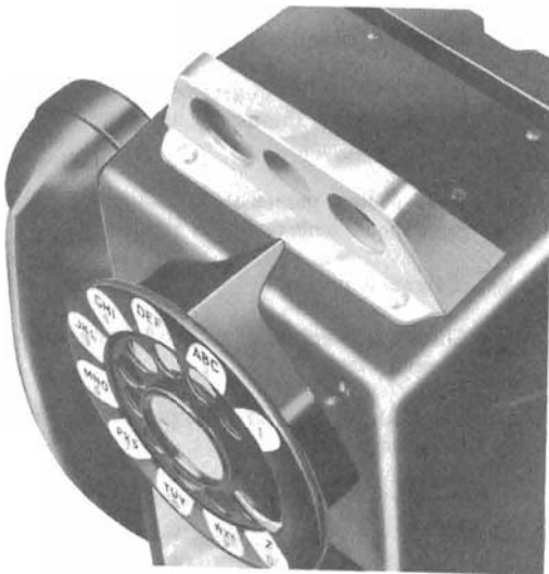
Fig. 30—P-14A544 Coin Deflector in Place
