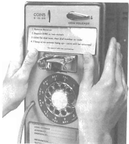
Fig. 12—Installing Instruction Cards (1A-Type)
